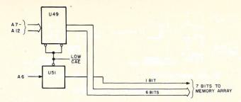
Fig. 2. Address path during Column Address Enable.
